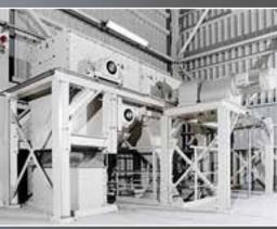
Discharge section of a WB 640 with 30 kW drive
