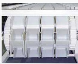
Multiple bucket belt at the tensioning unit
