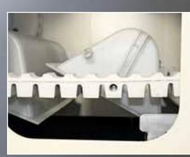
Buckets are emptied by the tilting mechanism
